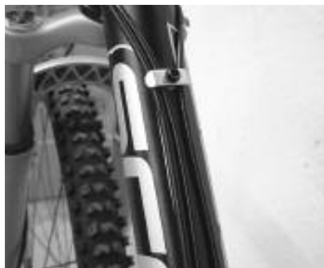
Smart Cable Routing
