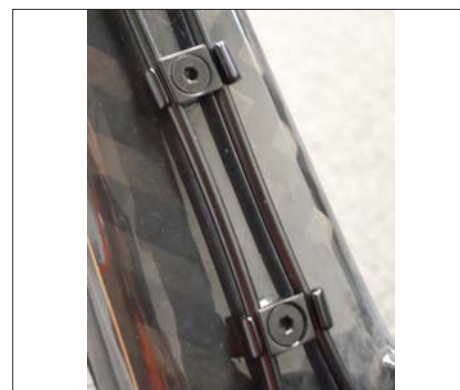
Smart Cable Routing
