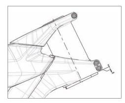
4. tighten the 3 screws with 5Nm/44in-lbs
