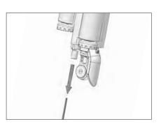
4 remove the old cable by pushing/ pulling it out from the TWINLOC lever
