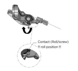
Cut the cable 5mm behind the roll and secure it with a cable end-cap.
