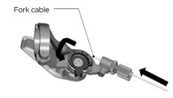
and secure the cable by fixing the 2mm allen screw with a tightening torque of 0.9Nm/ 8lb/in as shown on the drawing below on the roll.
