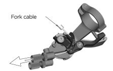
Fix the cable with the 2mm allen screw on the barrel adjuster on the fork crown with a tightening torque of 0.9Nm/ 8lb/in, cut the cable and secure it with a cable end-cap. Please refer for this action also to the manual of SRAM/RockShox attached to the bike.
