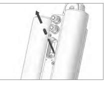
remove the end cap of the cable 2 with pliers
