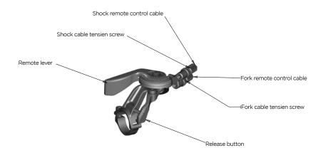
Please note that the cable for the rear shock is ALWAYS the upper cable on the lever as shown in drawing below.
