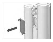
Remove the cap of the cable housing window on the shock by turning the screws counter clockwise using a 1.5 mm allen key
