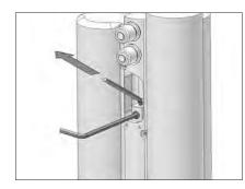
6 tighten the cable and fix the cable fixing screw (S10) by turning it clockwise with a 2.0 mm allen key and a max. tightening torque of 1.6 Nm
