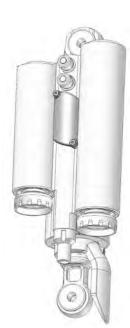
9 remount the cap of the cable housing window on the shock by turning them clockwise using a 1.5 mm allen key and a maximum tightening torque of **0.3 Nm**
