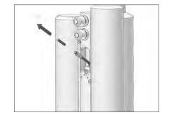
**8** push the "open-ended" cable cap on the cable until it touches the cable sled, fix it by squeezing it with pliers and cut the cable just above the cap
