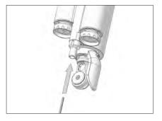
5 insert a new cable via lever hole and cable housing and push it into the shock as shown
