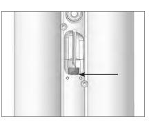
to double check accurate cable tension please push the TWINLOC lever to "TRACTION-MODE". The mid of the cable fixing screw (S10) should be at the edge of the lower cable housing window on the shock. For fine-tuning please adjust the cable tension via the barrel adjuster (L4) on the TWINLOC lever.
