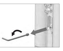
3 loosen the cable fixing screw (S10) by turning it counter-clockwise with a 2.0 mm allen key
