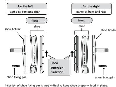
Insertion of shoe fixing pin is very critical to keep shoe properly fixed in place.
