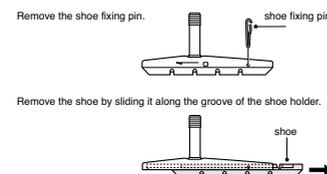
There are two different types of shoe and shoe holder to be used in the left and right positions respectively. Slide the new shoes into the grooves on the shoe holders while taking note of the correct directions and pin hole positions.
