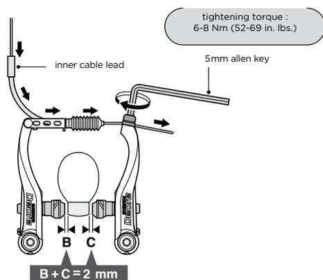
3. Adjust the distance with the spring tension adjustment screws.
