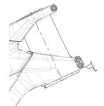
4. tighten the 3 screws with 5Nm/44in-lbs
