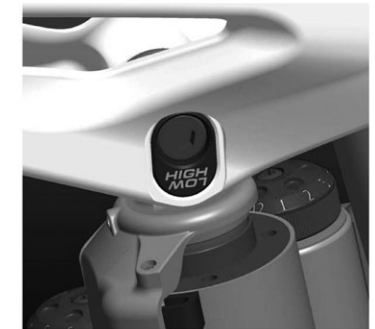
HIGH Setting, hohes Tretlager
