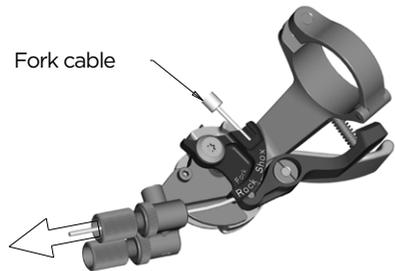
Fix the cable with the 2mm allen screw on the barrel adjuster on the fork crown with a tightening torque of 0.9Nm/ 8lb/in, cut the cable and secure it with a cable end-cap. Please refer for this action also to the manual of SRAM/RockShox attached to the bike.
