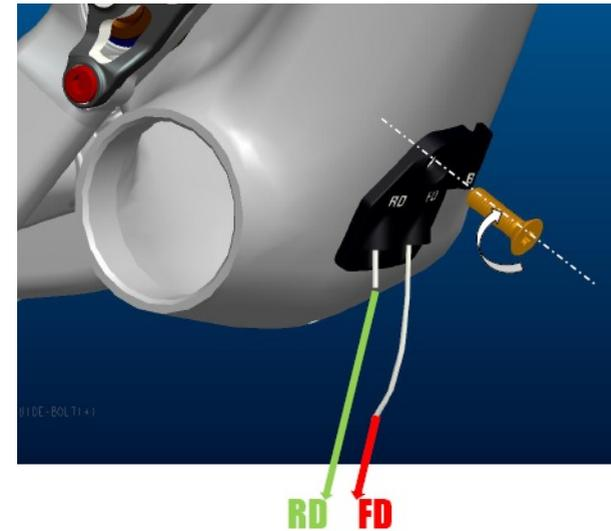
Push the outer cable housings on the cables into the cable guide but make sure to respect the needed length as shown in the next drawing!
