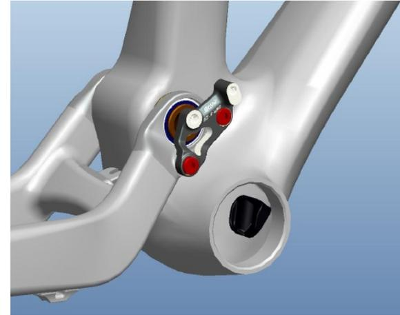
All alloy front frames of Spark have a BB shell for 73mm BSA standard.
