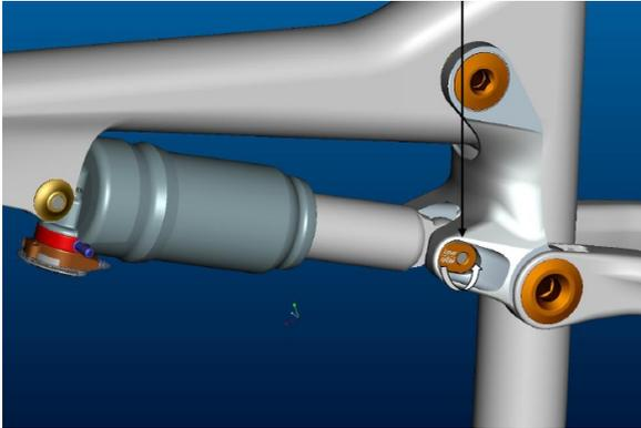
1. low BB for lower center of gravity over ground
