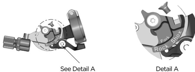
To assemble the cable please bring the lever into the All Travel Mode, push the cable into the lever-eyelet as shown on drawing below, push it through the pre-cut cable housing and fix it at the assembly unit on top of the right side of the fork crown.
