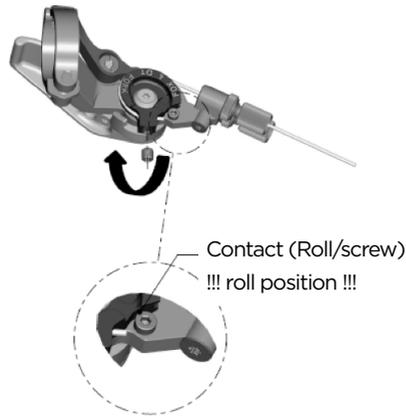
Cut the cable 5mm behind the roll and secure it with a cable end-cap.
