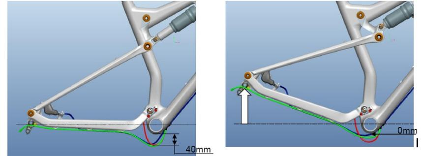
For the rear brake please assemble the cable as shown in the following drawings:
