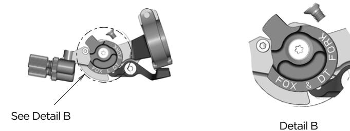
To assemble the cable please bring the lever into the Full (Travel) Mode
