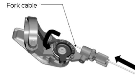
and secure the cable by fixing the 2mm allen screw with a tightening torque of 0.9Nm/ 8lb/in as shown on the drawing below on the roll.
