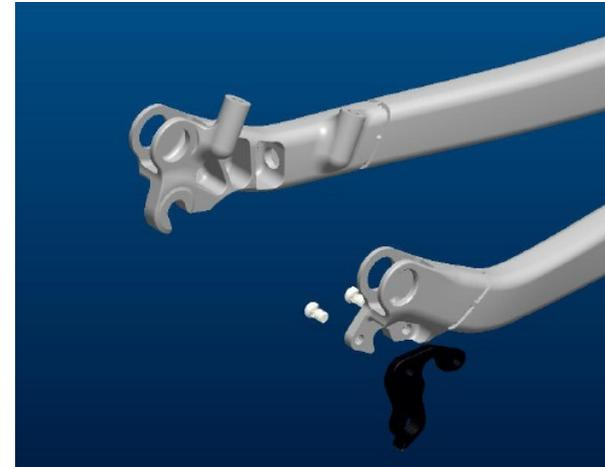
The replaceable hanger is available via the Scott distribution with parts number 206473.
