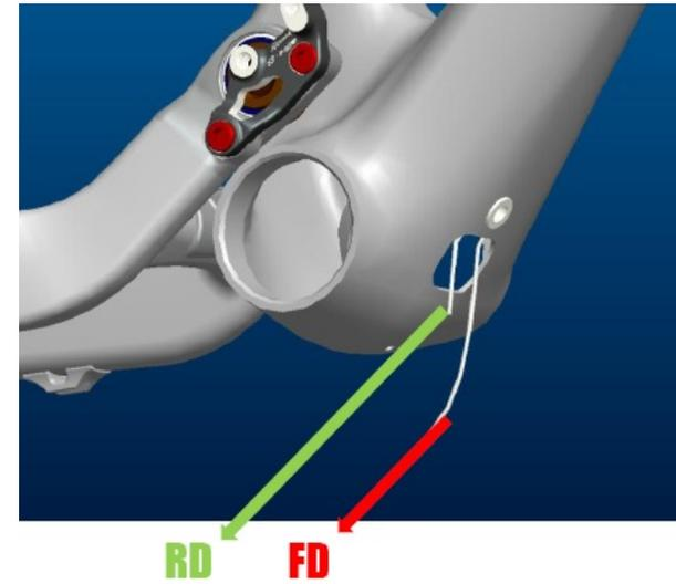
Push the cables through the cable guide as shown below and fix the cable guide on the downtube with a 3mm allen key and a tightening torque of 4Nm/35in/lbs
