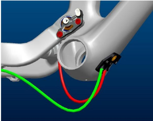
Please make sure to respect the 40mm distance between the cables and the BB (bottom bracket) housing to avoid “ghost-shifting” and/or damages on the shift cables and brake hoses.
