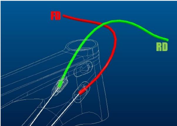
Please note that the inner cables need to cross each other 1 time on the inside of the downtube before you pull them out through the cable slot on the lower downside of the downtube.
