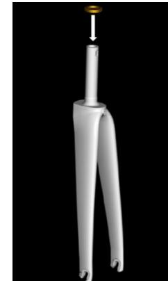
1. Assembly lower bearing on fork carbon crown
