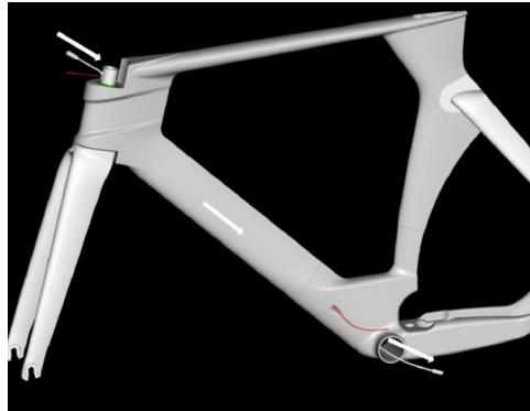
6. Push the brake cable outer housing along the brake cable all way upward from the BB to the steerer tube holes into the frame
