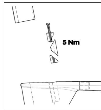
In case the seatpost was cut too short or another rider wants to adjust the seatheight but keep the seatpost maximum inside the seatpost pocket you can use the adapter-set as shown below to adjust the length of the seatpost individually.
