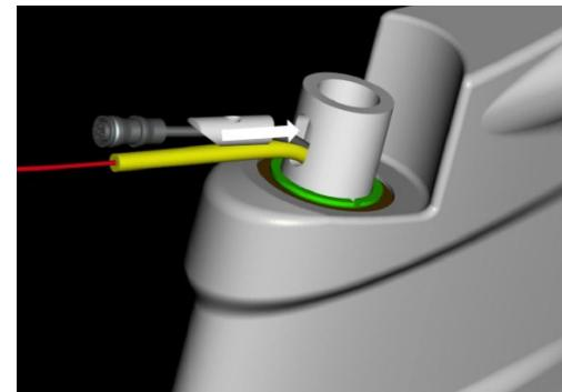
8. Assemble the stem main body with its rear cap on the steerer tube
