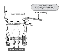
3. Adjust the distance with the spring tension adjustment screws.
