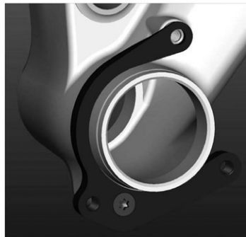
Use 1x 15mm long bolt. Top hole is secured by chain device bolt. Not for use with guides with bashplate mounted on ISCG boss.
