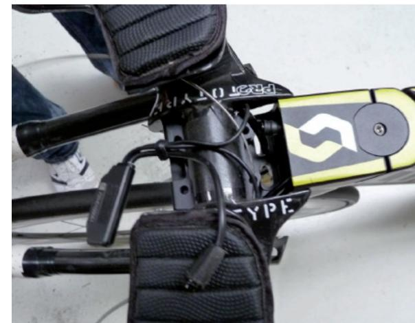
12. Connect the Di2 wire plugs and finalize the assembly of front and rear brake cables
