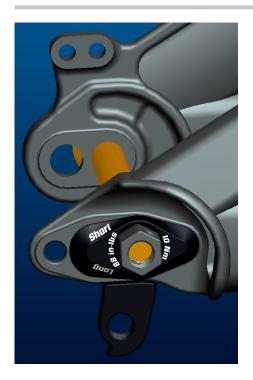
The Gambler 700 offers the possibility to change the drop out hanger in case of damage, but you also can choose between 2 different rear-axle positions which results in 2 different wheelbases.
