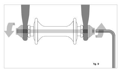
Hex nuts or hex key bolts which are threaded on to or into the hub axle (bolt-on wheel, fig. 10)
