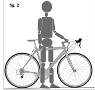
you'll ride on unpaved surfaces should give you a minimum of three inches (7.5 cm) of standover height clearance. And a bike that you'll use off road should give you four inches (10 cm) or more of clearance.
