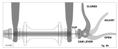
A hollow axle with a shaft ("skewer") running through it which has a nut on one
