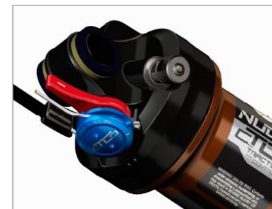
3. tighten the cable and fix the cablefixing screw (S7) by turning it clockwise with a 2mm allen key and a max. tightening torque of 1.6Nm.
