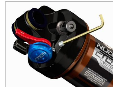
2. insert a new cable via lever hole and cable housing and push it into the shock as shown around the remote wheel (S6).
