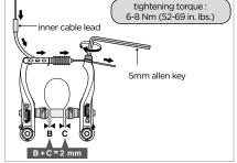
3. Adjust the distance with the spring tension adjustment screws.
