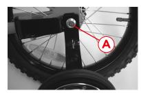
2. Put part B in part C and fix it with nut A with the washer between nut A and part C
