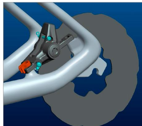
The rear disc brake on Scale is Postmount (PM) Standard on the left chainstay and optimized for 160mm/6" rotors, so the calliper can be mounted directly without adapters on the Postmount fixation.
