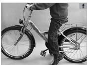
Special attention should be paid to the adjustment of the control elements, such as brake levers. Easy reach and operation should be ensured for the child (a).
