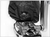
Make sure that the pedals and shoe soles are always clear of mud and other foreign bodies and grease the lock-in mechanism with lubricant at regular intervals (a).
