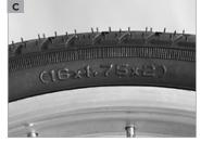
If you want to mount a new tyre, you need to observe the sizing system and the actual size of the old tyre. The latter is specified in two different units on the side of the tyre. One of the sizes is the standardised size in millimetres which is more precise, e.g. the number sequence 47-305 means that the tyre is 47 mm wide when fully inflated and has an inner tyre diameter of 305 millimetres. The other size is indicated in inches (e.g.  $16 \times 1.75 \times 2$ ) (c).
