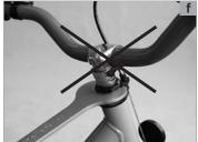
Now you can move the handlebar/stem-unit up and down as a whole. Be sure not to pull out the stem too far. The mark on the stem (end. min. max. stop. limit or the like) should always remain within the tube (a). Setting the stem to a lower position can only add to your safety!
