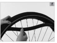
To make sure the inner tube does not get pinched between the rim and the bead, move the tyre sideways back and forth between the sides of the rim. While doing so, also check whether the rim tape has shifted.
