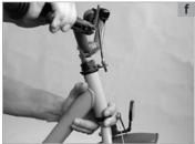
To check whether the headset runs smoothly, lift the frame up until the front wheel no longer touches the ground. The handlebars should turn from far left to far right without feeling roughness or tightness at any point. With a gentle tap on the handlebars (a) the fork should turn easily from the middle position.
