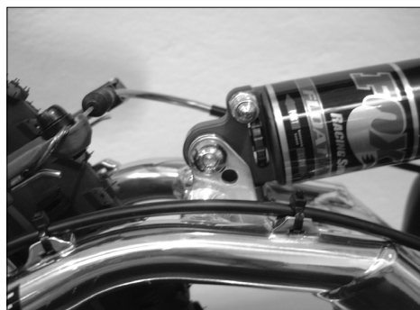
85mm, 10mm lowered BB, for XC
