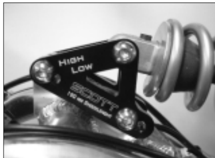
adjustment-plates for different lengths of suspension.
