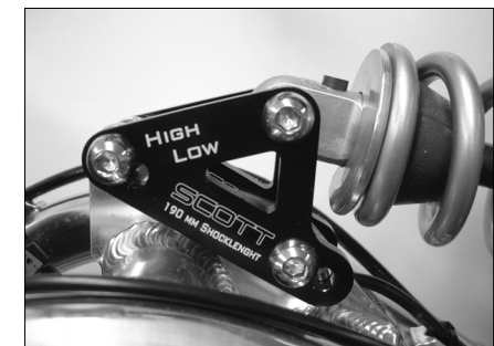
adjustment-plates for different lengths of suspension.
