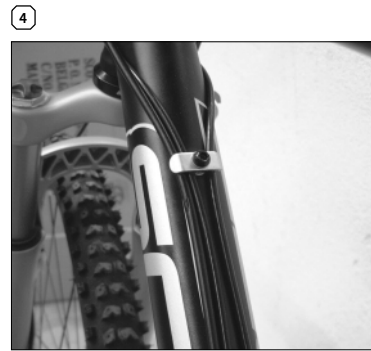
Smart Cable Routing
